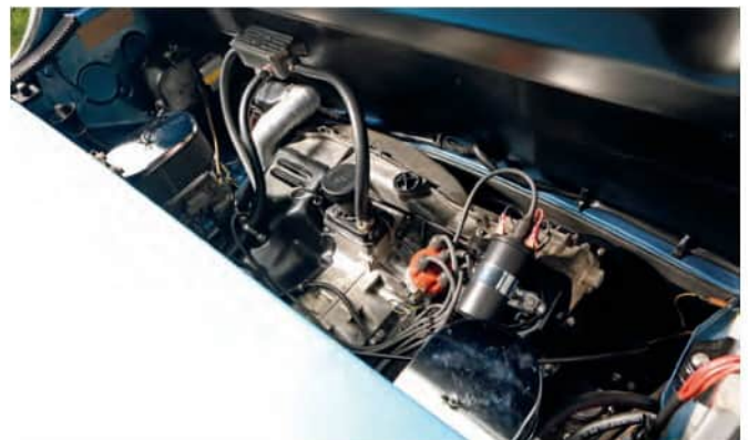
Clockwise, from main: as a 1974 model, Darren's 914 has Federal 'bumper impact-protection guards'; 2-litre engine was the biggest 'four' offered; Fuchs alloys; stock injection has been replaced by carbs
