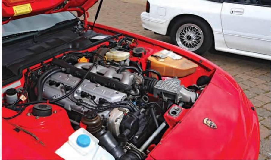
Porsche's 3-litre, 208bhp 'four' uses 104mm bores with cast rather than forged pistons for less weight
