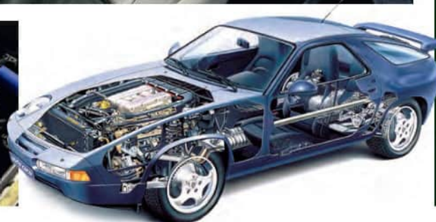
From top: funky Pasha trim is more in keeping with the 928's character than leather. Below: quad cams from S4; cutaway shows transaxle layout
