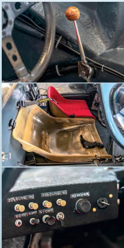
From top: gearknob is turned from balsa wood; glassfibre bucket seat's padding was removed to give a touch more room; dashboard switchgear's labels remain authentically of the period
