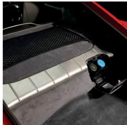
Workmanlike cockpit of the Porsche; flap in the mid-engined Cayman's luggage area gives access to fluid reservoirs; smaller 17in alloys fitted to this car
