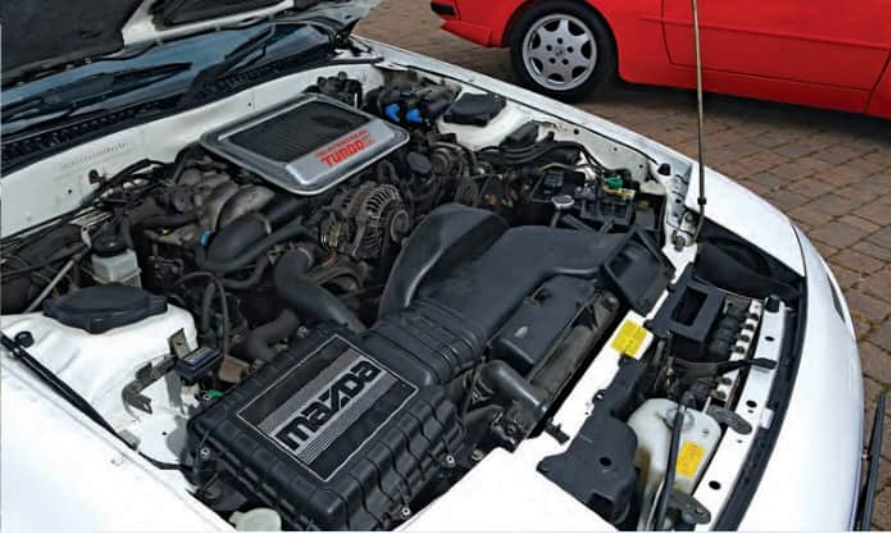
Lighter rotors, higher compression and sharper engine management upped Turbo II's output to 197bhp
