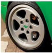
From top: window-hugging 935-style door mirror; Ruf-badged VDO dials – sticker on speedo warns you not to exceed 300kph; Speedline alloys (17in here) got bigger over the years while tyre profile shrank
