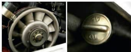
Fan cools motor; check oil level with engine running
