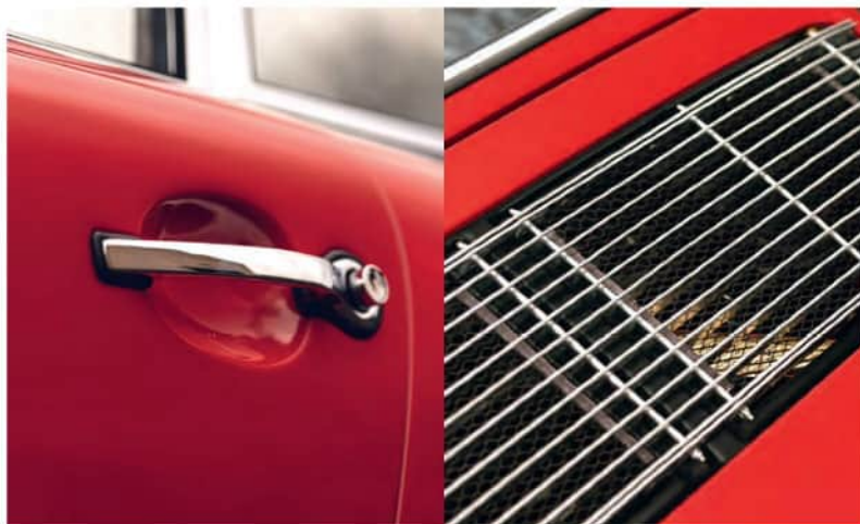
Above, from left: pushbutton handles are slightly different to those on later cars; sharp engine-cover slats sent the designers back to the drawing board
